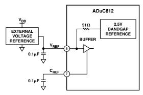
Figure 10. Using an External Voltage Reference
